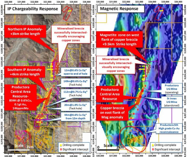
Figure 1- Selected extensional drilling results, magnetic and IP chargeability response of the Productora mineralised system- +9.5km in strike length.
