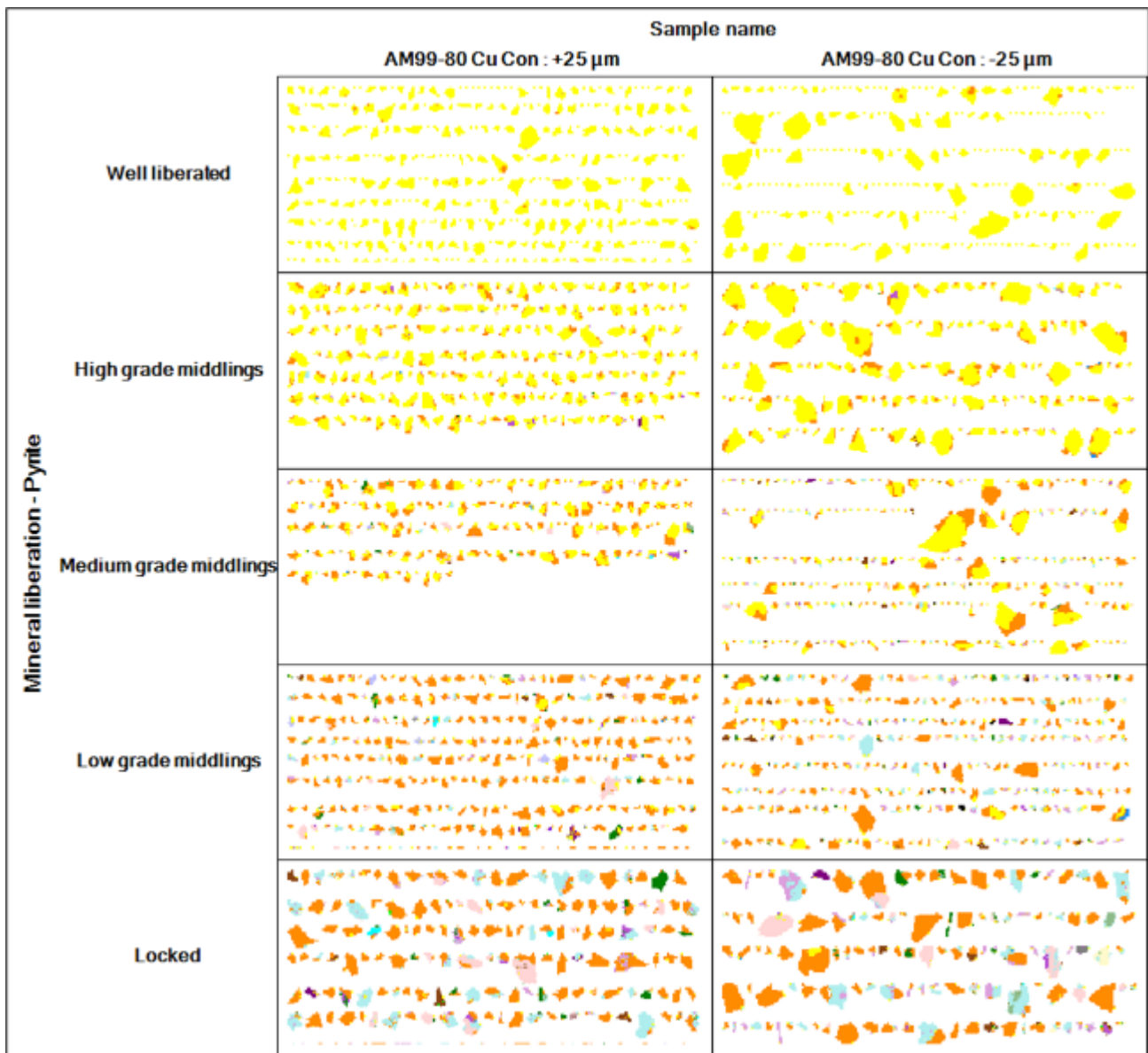
Figure 13.64 : Open Pit Production Feed – Pyrite Liberation in Copper Concentrate
