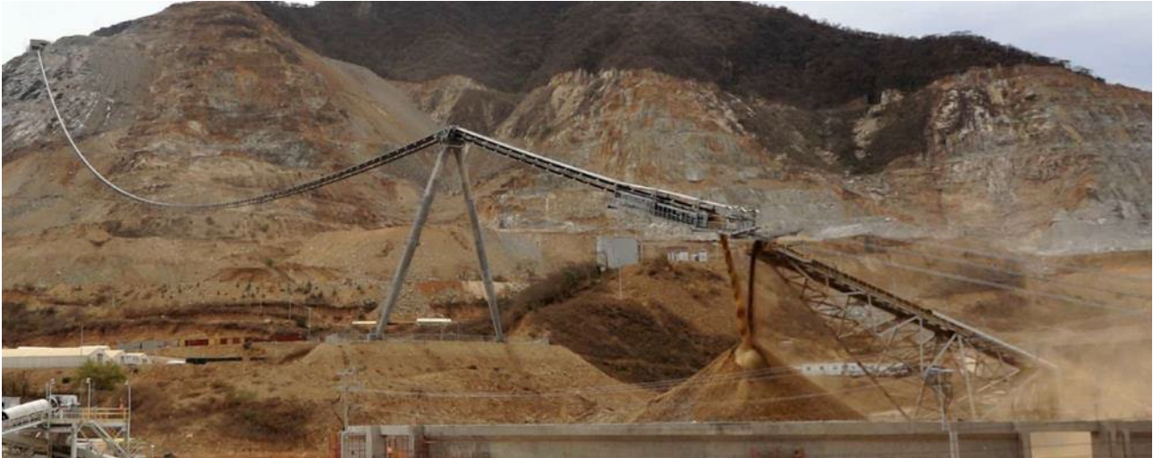
Figure 18.6 : RopeCon installation to transport material from the crusher installation on the bluff to the plant stockpile at El Limon, Mexico.
