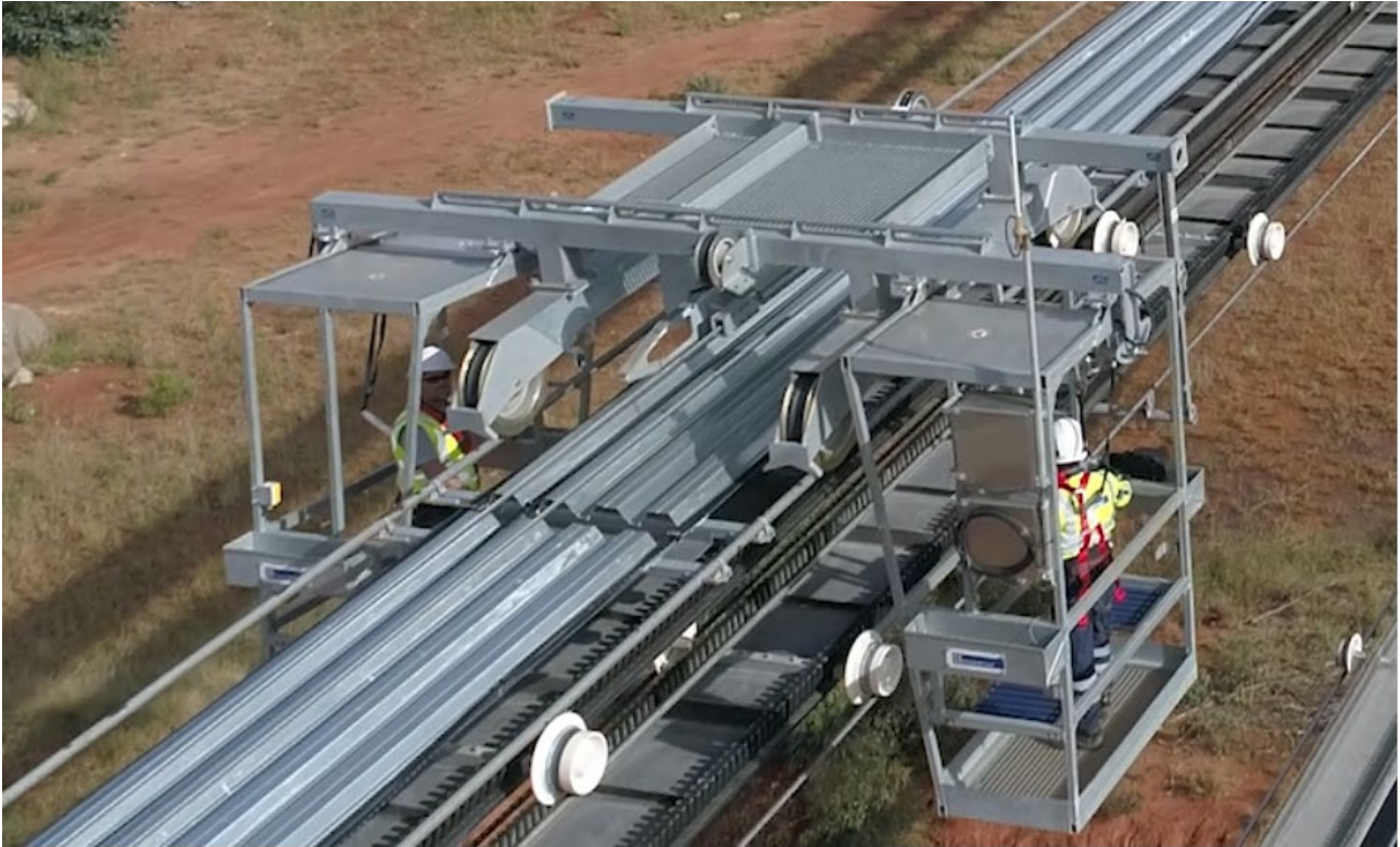
Figure 18.7 : RopeCon Inspection Carrier in Operation at Booyensdal North, South Africa.
