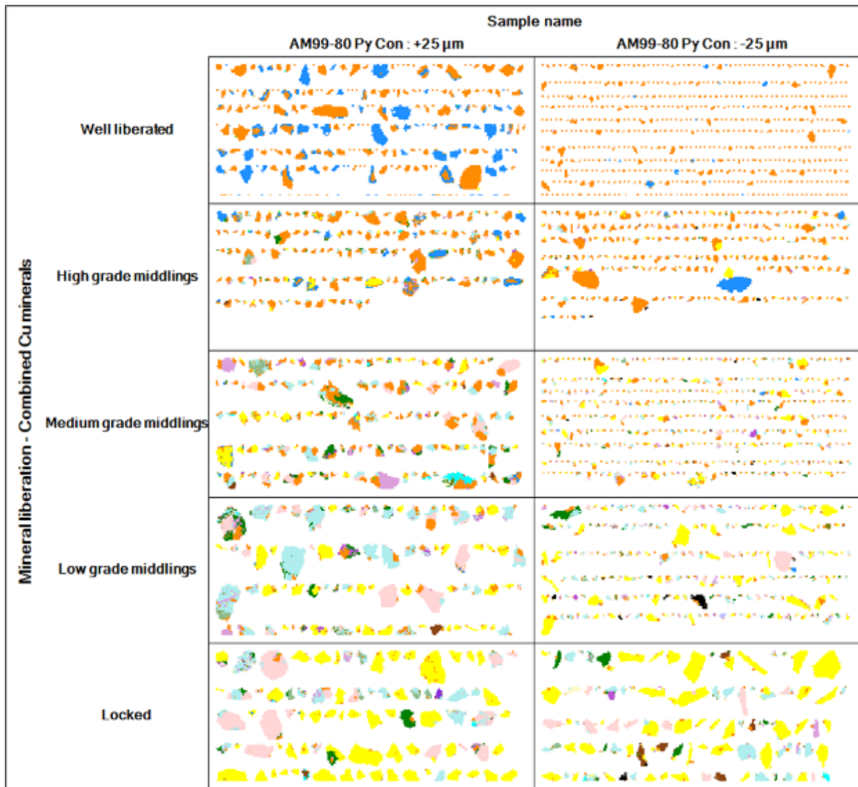
Figure 13.68 : Copper Mineral Liberation in Pyrite Concentrate
