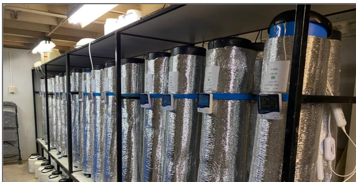
Figure 3. Novaminore® 1 m Column Leaching Test on Productora Oxide material
