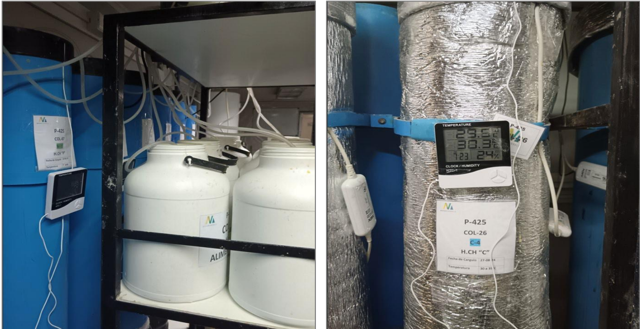
Figure 13.20 From Left to Right: Conventional Leach Column and NOVAMINORE Column
