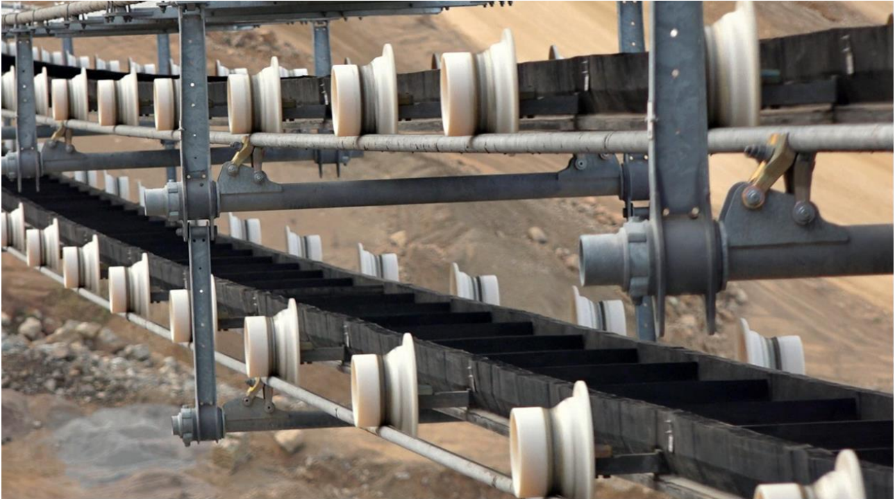
Figure 18.21 Close up view of Rope Conveyor belt with corrugated side walls and track system
